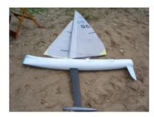
single mast position was blown apart by making a lash-up 'C2' Stollery Swing Rig with a polythene rig bag for the mainsail on Geoff Smale's 'Kiwi Magic' that came with no smaller rigs. He had no problem using this second suit whereas those with 'Crazy Tube's and the same rig had real problems in tacking and accelerating after the tack. The mast position on Geoff's boat was a few inches further forward and demonstrated how important this was for making
