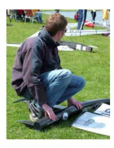
Tube Too' demonstrated the reaching and marginal planing ability of an even narrower, totally circular sectioned hull with a maximum diameter of 118mm, a displacement of 4.8kg and a draught of 617mm"
